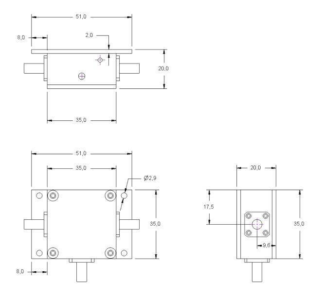
Note1 : All measures in mm. Tolerance : 0.1 mm.
