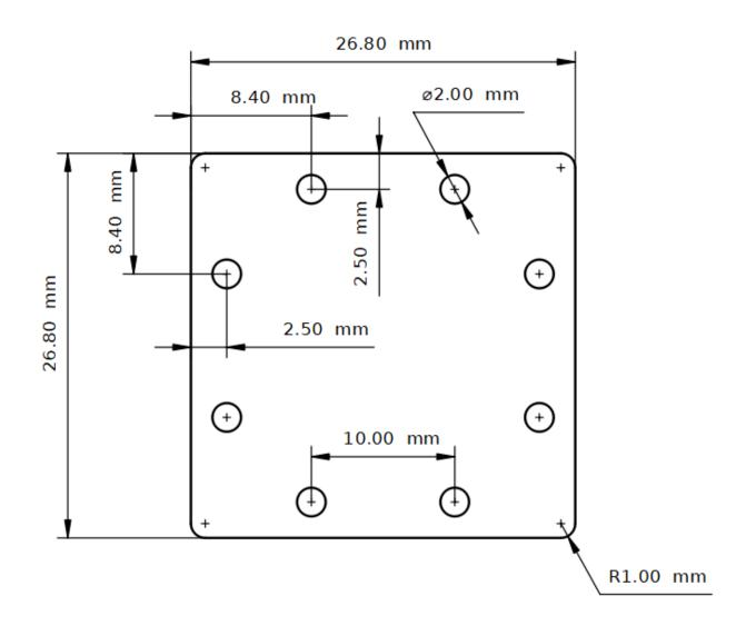
Note1 : All measures in mm. Tolerance : < 0.1 mm.
