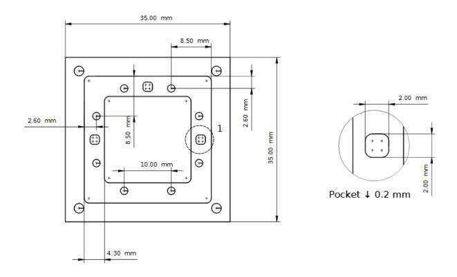
It also shows a small pocket located near each SMA port. It can be used by the designer to reduce the impedance of the SMA landing area. This feature was added during 2024.
