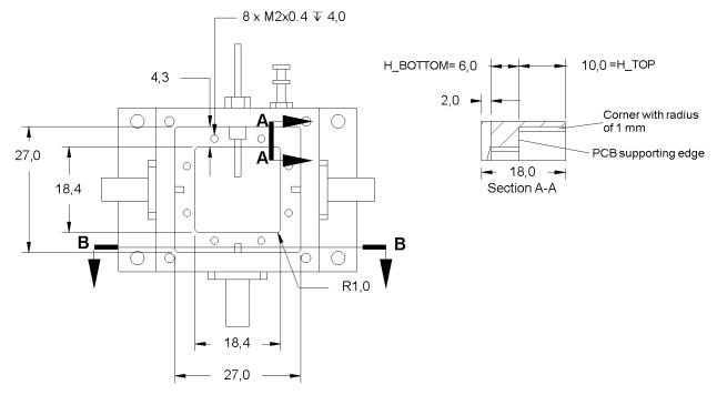
Distances PCB mounting frame and SMA connector pin
